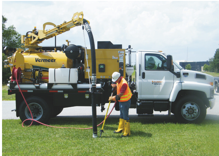
With its positive displacement blower rated at 1,200 cubic feet per minute, the Xtreme product line takes the combination air/water vacuum excavation technology to the next level, says McLaughlin president Dave Gasmovic.
